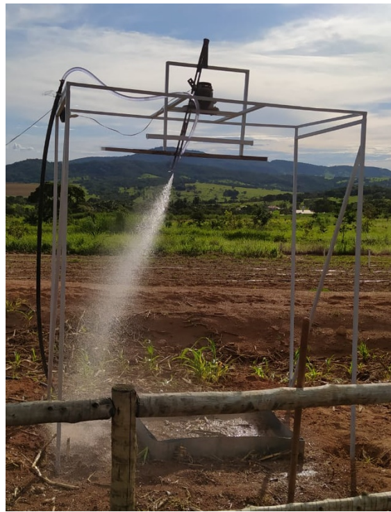
FIGURE 4. Rainfall simulator assembled for the sprinkler nozzle uniformity test.
