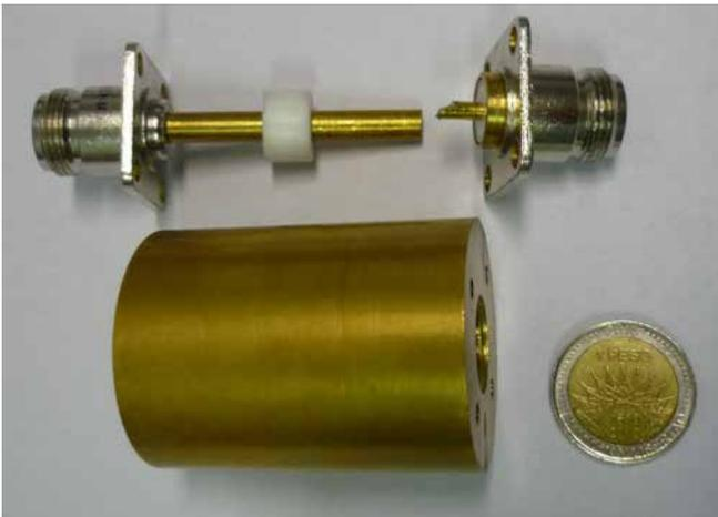
Fig. 11: Sample holder with the inner and outer cylindrical conductor, a Teflon sample with  $d = 8$  mm and two connectors.
